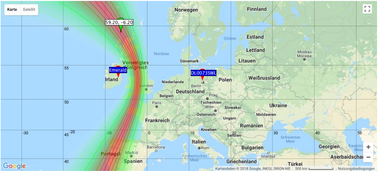
Figure 4: Each pair of receiver will draw a hyperbole onto a map – a curve of all possible positions of a transmitter, matching the same “time difference of arrival” of this pair. Here an example with receivers “Emerald” and “DL0073SWL” on 198 kHz (BBC4), July 25 th , 2018, 09:30 UTC.
