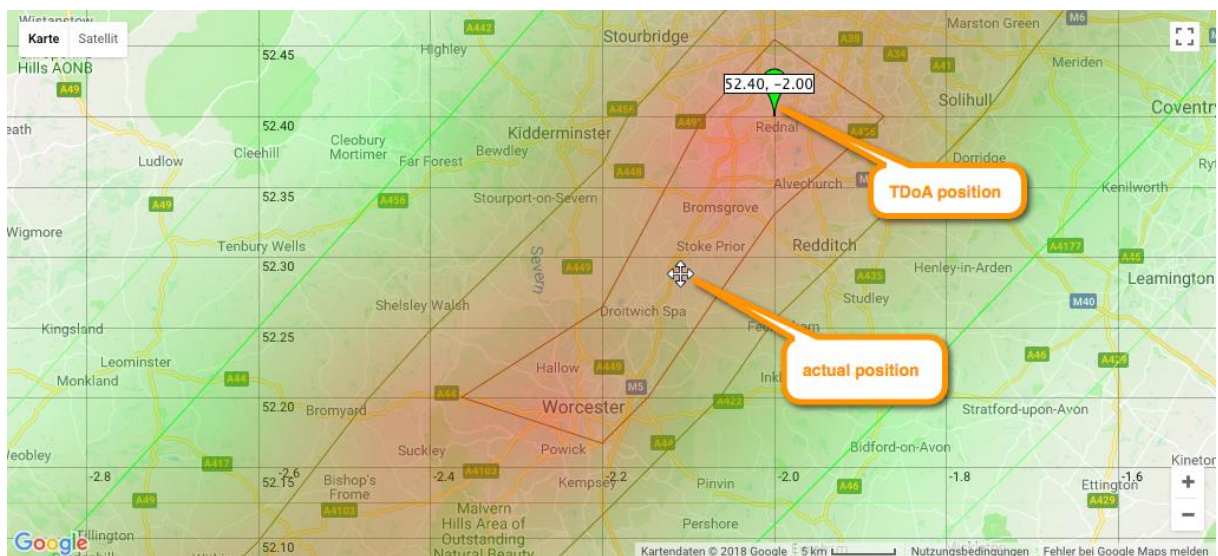
Figure 7: ... with the most likely location of the transmitter duly marked. In this case with a deviation of just < 10 km south-west.
