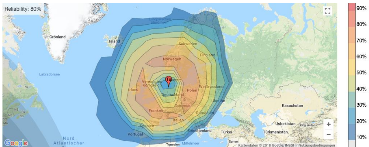
Figure 9: Judging from the stable reception, the transmitter should be most likely located in a zone of 70 % base circuit reliability.
