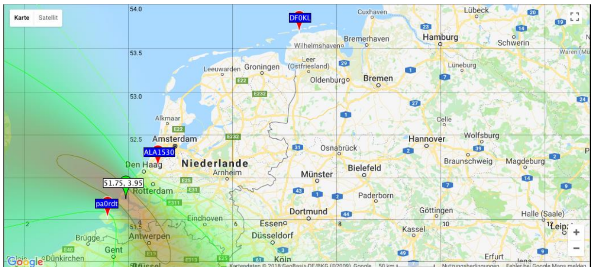
Figure 22: By the aid of two other receivers nearby, the actual location on Goeree Island is nearly exactly hit.
