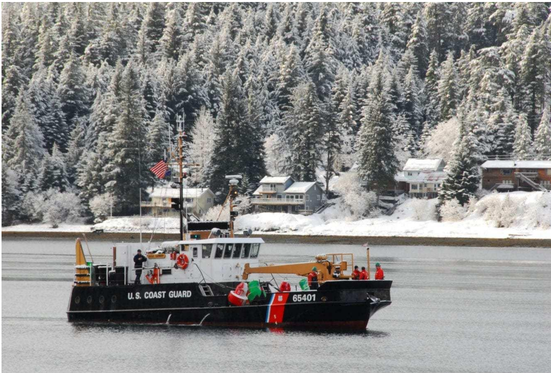
Crew members aboard the Coast Guard Cutter Elderberry, a 65-foot inland buoy tender homeported in Petersburg, Alaska, prepare buoys to be set in the Gastineau Channel.
